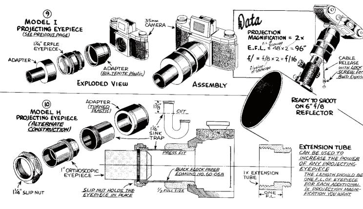
the 1x position and the afocal position it is possible to obtain a complete range of magnifications, from no magnification to infinite magnification--all with a lens adjustment of less than one focal length, Fig. 4.
