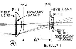
I-I-I RAMSDEN IS CORRECTED FOR LATERAL COLOR BUT EYE RELIEF IS ZERO,...DUST CAN BE SEEN ON FIELD LENS WHICH COIN-CIDES WITH IMAGE PLANE
