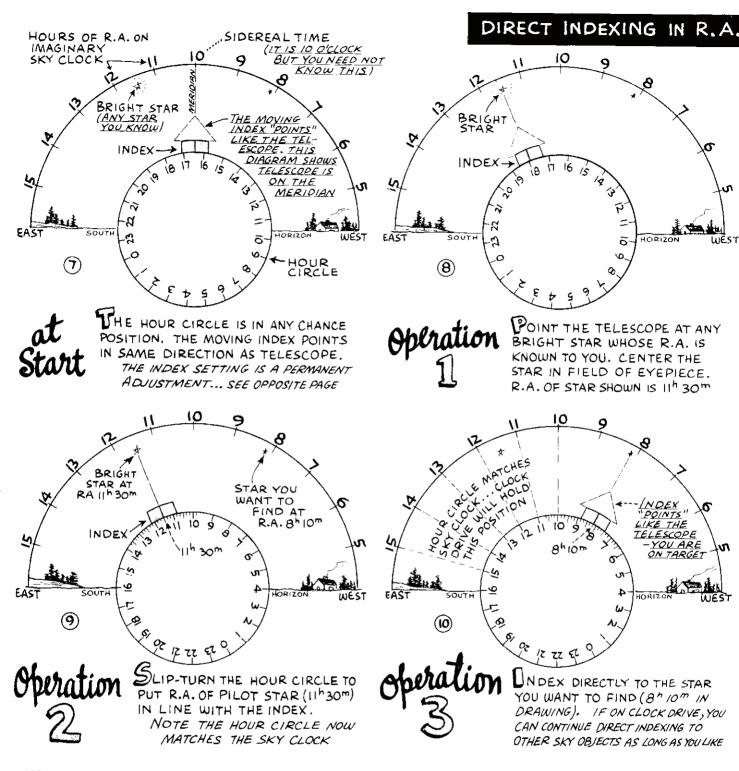
INDEXING BY HOUR ANGLE. In this familiar method of star-finding, the  $R_{\cdot}A_{\bullet}$  of the star is subtracted from sidereal time at the moment. The result is the hour angle of the star from your meridian. The most convenient scale for setting off an hour angle is the 0-6-0-6 scale, with one of the zero marks set to the meridian. This method is cumbersome and time-consuming--you use it when you have to, but otherwise you are miles ahead with direct indexing.
