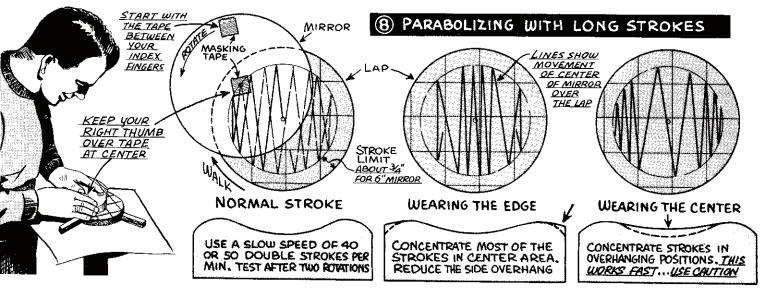
LONG STROKE PARABOLIZING. The actual work of parabolizing from a sphere or nearsphere is done with a stroke of maximum length and sidewise zig-zag, Fig. 8. Under good conditions you can parabolize a 6-inch f/8 in as little as five minutes. However, it is best to stretch the work over a longer period of about 20 minutes, using a slightly shorter stroke and less side overhang.
