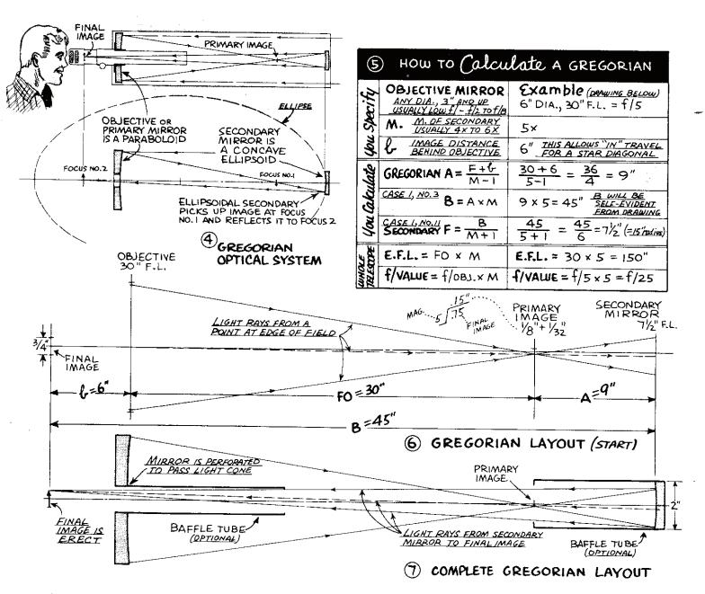
larges the primary image. So defined, a Newtonian is a simple reflector rather than a compound one. The Gregorian and the Cassegrain are the two basic compound reflectors.
