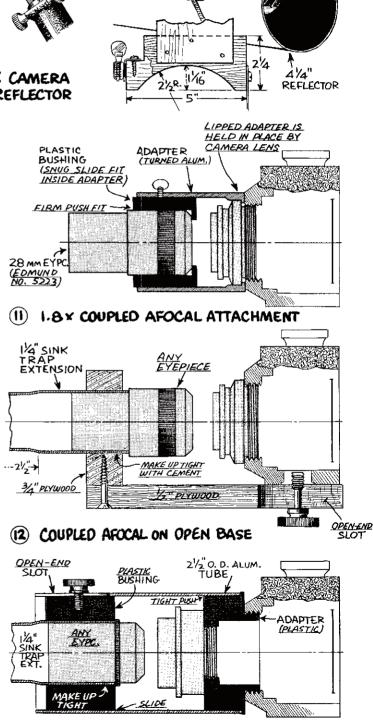
(3) COUPLED AFOCAL WITH 3" F.L. CAMERA LENS
