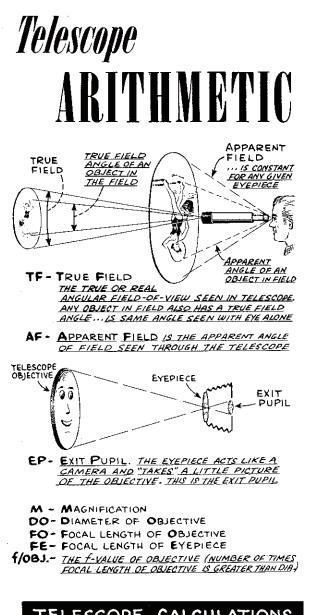
ONE OF THE first things you learn about telescopes is that the magnification is equal to the focal length of the objective divided by the focal length of the eyepiece. This basic calculation is No. 1 in the chart below. Like all equations, it can be transposed, as shown by formulas 2 and 3. No. 2 determines the f.l. of eyepiece (FE) needed to obtain a certain magnification; No. 3 gives the f.l. of objective if M and FE are known.
