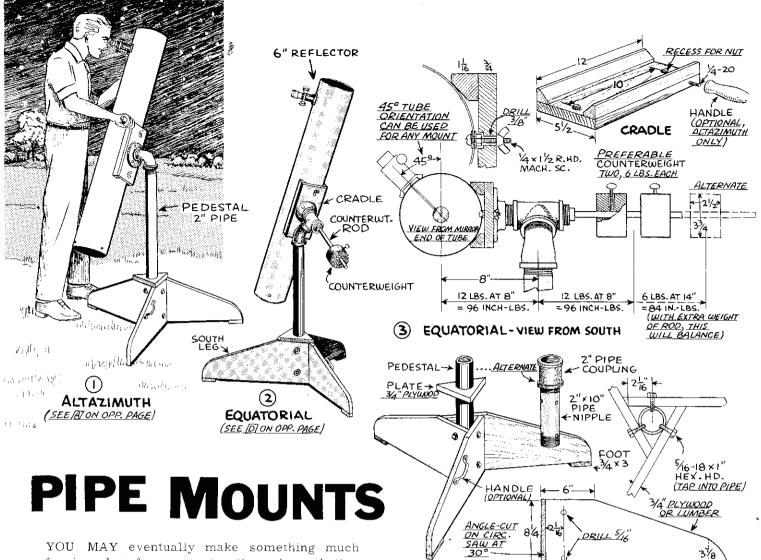
YOU MAY eventually make something much fancier, but for a starter there is no better telescope mount than the turn-on-threads variety made of pipe fittings. With this kind of mount you get the needed mechanical movements by simply leaving the pipe fitting a little loose, free to turn. Much the same construction is used for both altazimuth and equatorial mounts. Both have two axes at right angles, but the primary axis of the altazimuth stands erect, Fig. 1, while the equatorial is tilted, Fig. 2.
