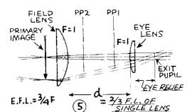
1-1-33 RAMSDEN IS STOCK DESIGN WITH LENSES SAME F.L. AND SPACE 33 F.L. OF SINGLE LENS. SPACING LESS THAN 1/2(F+F) CAUSES LATERAL COLOR
