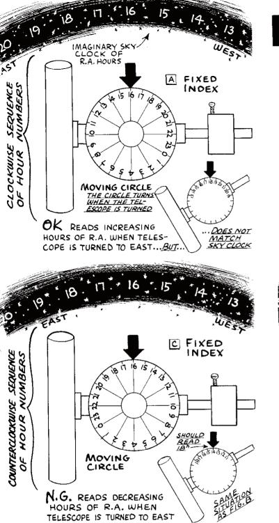
numbers on the hour circle would not match the imaginary clock in the sky. The other two systems do not work at all--they simply do not index or point the telescope the right way. However, even these arrangements can be used to set off an hour angle.
