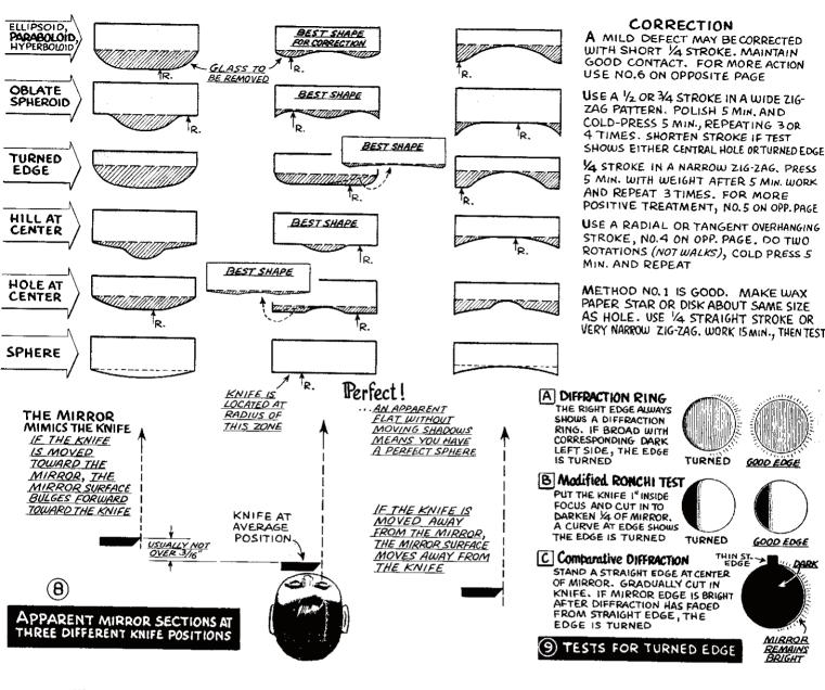
with no light at all, you have a real-for-sure turned edge. Fig. 9B shows one of the more popular tests; it works only when the light source is a slit. In applying Fig. 9C test, you must hold your head steady, eyes straight ahead, avoiding any tendency to sneak your gaze around the edge of the knife.
