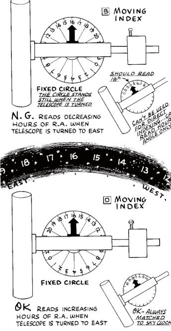
cope. The fixed hour circle has movement in that it can be slip-turned as desired. If a clock drive is used, the fixed hour circle is attached to the worm gear to partake of the clock movement, but it is still a "fixed" circle in that it does not turn when the telescope is turned. The clock motor itself should have counterclockwise rotation when viewed from the end of the clock shaft--this will drive the telescope in the required westerly direction.
