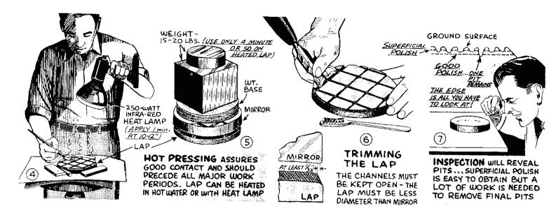
face sparsely charged. Each wet of rouge should be worked nearly dry since it is in this state that the rouge begins to wipe the glass with a vigorous polishing action. The drying mirror will become harder to push, and when it starts to stick and skip, it is time for a new charge of rouge. Polishing periods should be no less than 30 minutes--best to go an hour or more to get the frictional heat needed to allow the mirror to bed down snugly on its pitch pad.
