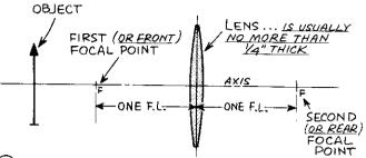
() LENSES ARE ASSUMED TO BE THIN. IF THE LENS IS THIN, A LINE THROUGH THE CENTER PROVIDES A REASONABLY ACCURATE REFERENCE PLANE FOR REFRACTION AND MEASURE-MENTS. THE PRINCIPAL PLANES SHOULD BE REFER-ENCE LINES IF LENS IS THICK
