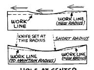
HOLE AT CENTER WORK LINE SHOWS GLASS TO BE REMOVED IF ORIGINAL RADIUS IS TO BE MAINTAINED. NORMALLY A SLIGHT CHANGE IN RADIUS IS PER-MISSIBLE ... WORK LINE IS THEN AS SHOWN IN RIGHT HALF OF DIAGRAM
