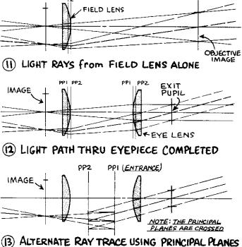
principal planes of the eyepiece as a whole and then draw light rays to the PP's, ignoring the lenses entirely except for the single item of diameter. The method of finding the PP's has already been described; the manner of making the drawing is as shown in Fig. 13. You draw a light ray to the image and keep right on going until you strike PP1. From PP1 to PP2, the ray is parallel to the axis. From PP2, the light ray goes to the corresponding part of the objective image, i.e., the exit pupil.
