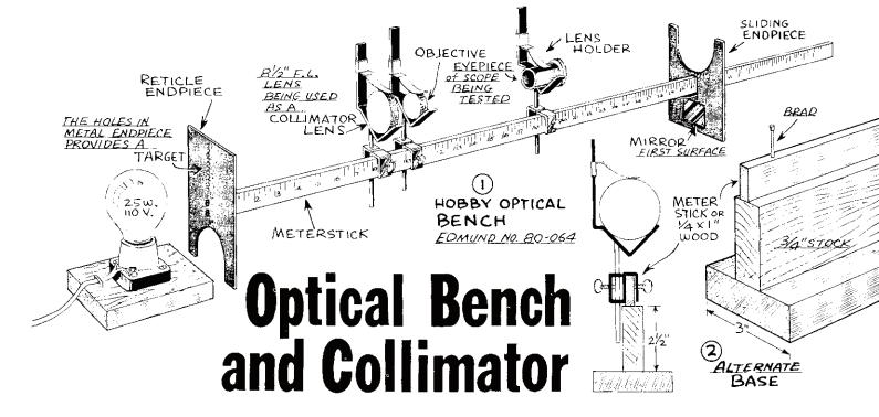
AN OPTICAL bench is the kind of equipment which may cost \$5 or \$5000. You can buy or build. Fig. 1 shows an inexpensive hobby optical bench you can buy. It is mounted on a wood meterstick. If you need a stronger or longer base, the construction shown in Fig. 2 can be used.
