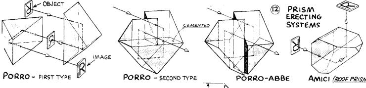
mate by the two-thirds rule, or you can determine air blocks exactly by making the simple bench test shown. The glass path itself of any prism is easily determined from a full-size drawing of the prism. Often the corners of a prism are cut off. When you are making a drawing, the corners should be restored to obtain the full side or hypotenuse from which the glass path is determined.
