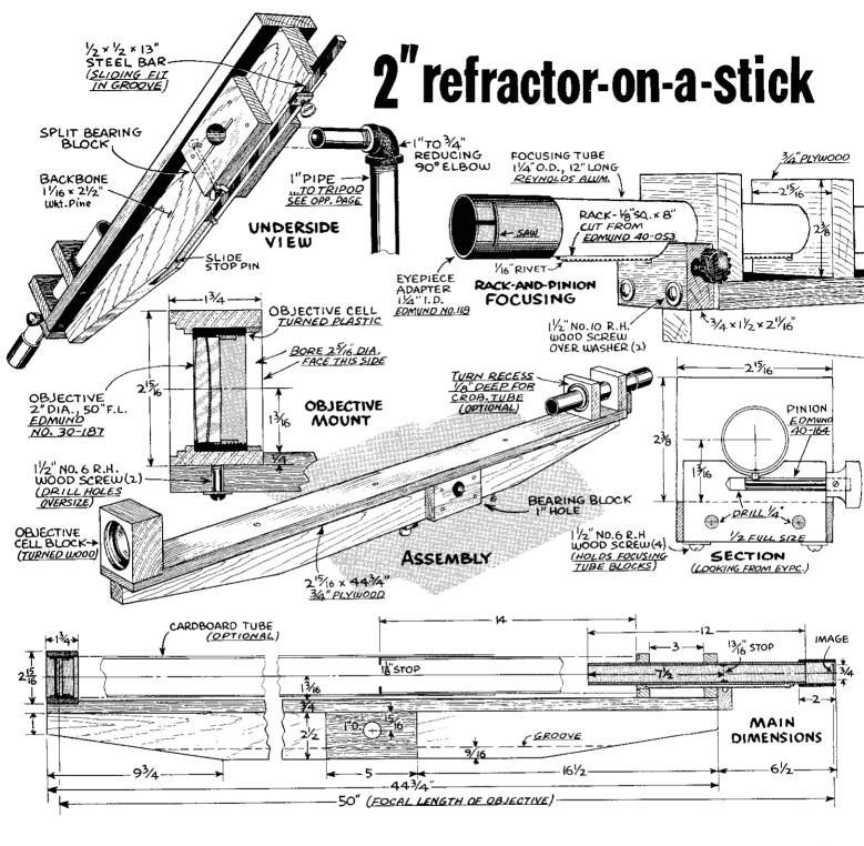
THIS IS a bigger version of the tubeless design shown on opposite page, with rack-and-pinion focusing added. The Edmund 2-in. objective is air-spaced, coated on all four surfaces, and is a good glass, assembled with three small bits of gummed foil (supplied) equally spaced around the glass. A sliding counterweight in the form of a bar of 1/2-in. square steel achieves a fair degree of balance around the altitude axis.
