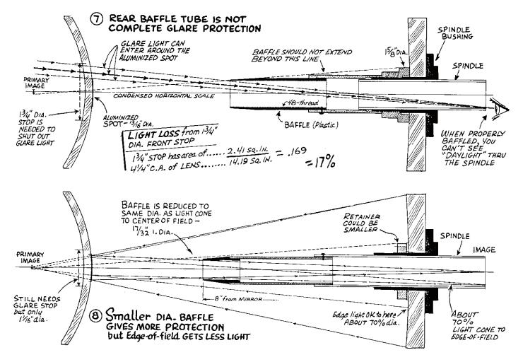
when properly installed. If you are buying a finished compound telescope of any kind, it is always wise to remove the eyepiece and look through the instrument. You should see only the secondary or its mounting; if you see "daylight" around the secondary or its mounting, you have a plain case of glare light. A little of this can be tolerated for astro use, but for the daytime scene you have to go all the way with 100% baffling of light outside the field of view.
