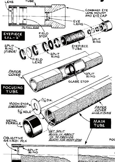
EDMUND simple lens telescope kit includes all the glass and parts to make an 8X astronomical refractor telescope. Of course the simple lens objective will show some false color and the image sharpnessis not the best. However, the scope is good enough to show craters on the moon in sharp detail, and it will reveal hundreds of stars not visible to the naked eye.
