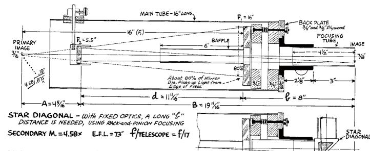
bit larger, specifically 5/32 inch for this design where the diameter of the image is 1/8 inch. With sliding primary, the extended erector tube is practically a full light baffle, making the objective stop less important but always worth fitting.
