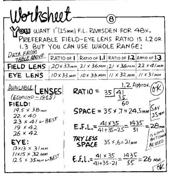
This construction is excellent for an erecting system or for a projecting eyepiece, but it is poor for ordinary telescope use in that there is no eve relief.
