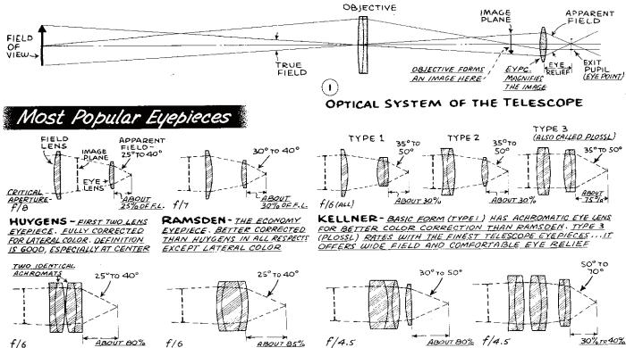
SYMMETRICAL-A POPULAR HOMEMADE STYLE. FOCAL LENGTH IS ABOUT ONE HALF F.L. OF LENSES USED ... IS GOOD ASTRO EYEPIECE
