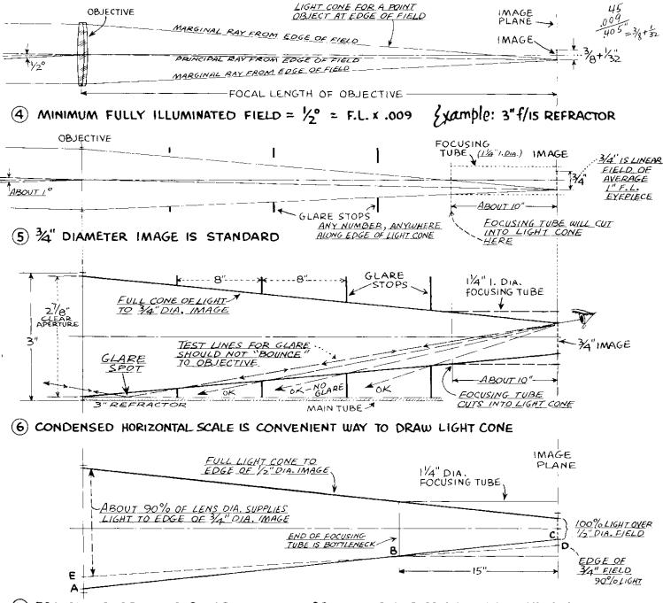
7) FOCUSING TUBE TOO FAR FORWARD WILL REDUCE THE SIZE OF FULLY-ILLUMINATED FIELD
