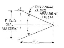
MEASURE THE ANGLE WITH A PROTRACTOR OR ADJUSTABLE TRIANGLE
