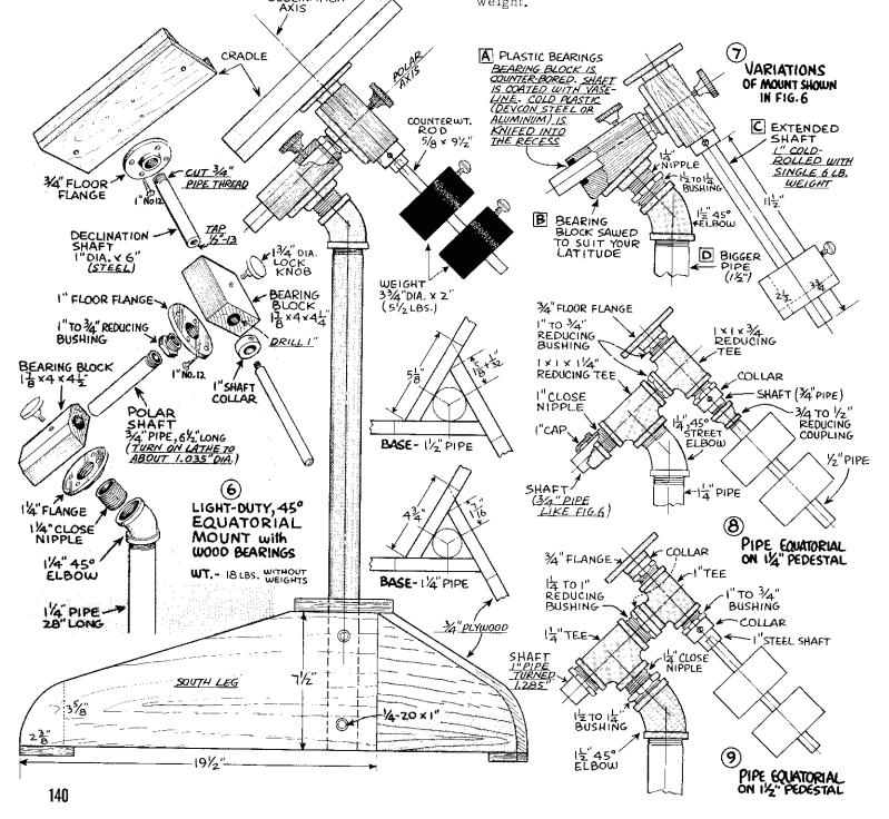
The only difficult part of making a pipe equatorial is the boring job, the 4 or 5-inch depth being near maximum for average home workshop equipment. An alternate is to rough-bore the bearings separately about .015 inch undersize, after which the assembly is made and the bearings hand reamed straight through to exact fit. Here again the required depth of cut is near the limit for ordinary reamers.
